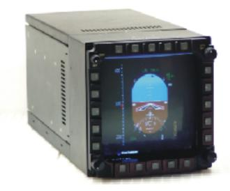
**Simulated** B-2 MDU **Multi-Purpose Display Unit** (ARINC-D)
